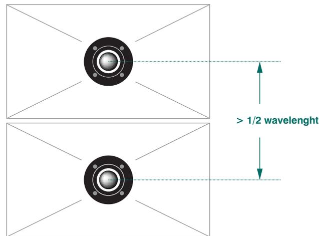
smallest HF speakers measures 24mm (so effective up to 4,1kHz), it is clear that this is not possible. Taking half the frequency (10kHz.), the required speaker size is still only 17,2mm. And we didn't even mention usable SPL with a speaker this size...!
