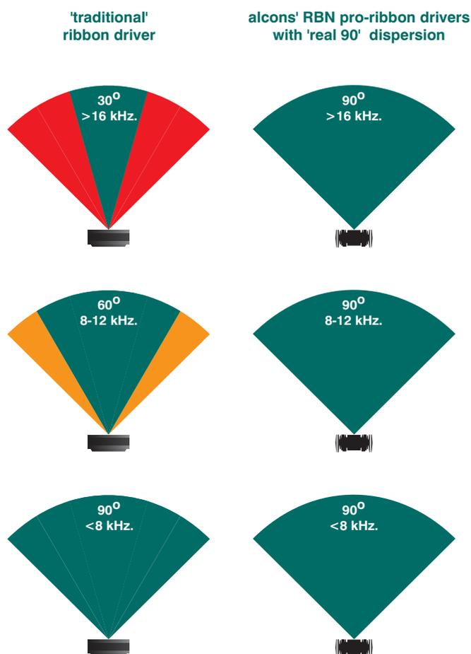
The RBN601 of the LR16 has a true power handling of 70W/1000W, enabled by the proprietary designed heat-management (patent pending) and an unsurpassed efficiency of 105dB (log average 2-10kHz 1W/1m on 90°x10° waveguide). The latest Alcons driver, the RBN1801, has a power handling of 210W/3000W and an efficiency of 110dB/1m (w/o waveguide).
