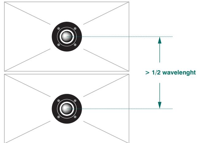
smallest HF speakers measures 24mm (so effective up to 4,1kHz), it is clear that this is not possible. Taking half the frequency (10kHz.), the required speaker size is still only 17,2mm. And we didn't even mention usable SPL with a speaker this size...!
