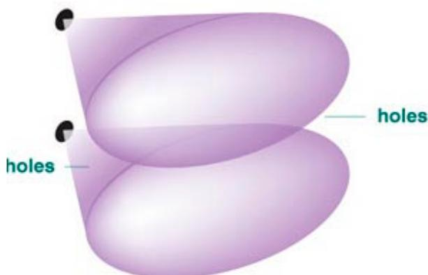
A pro-ribbon driver (a “flat diaphragm tweeter”) is by nature, a line source; A multiple of point sources generating planar sound waves, resulting in all natural cylindrical wave front.
