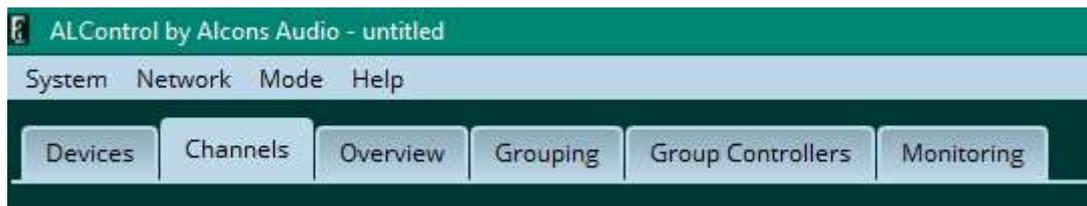
Channels: the selected Sentinel devices in the project form a list of channels. In this section, each channel can be configured with the required system factory preset (preset selector), the analogue or digital input signal and input channel. Each channel can also be configured with a manually selected name.
