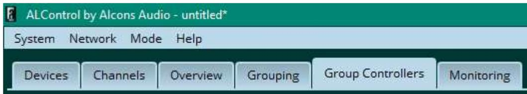
Group Controllers: resulting from the channel assignment, groups and sub-groups are formed that can be controlled in the “Group Controllers” Tab. The groups and sub-groups are visualized; This screen is visually free-configurable (drag & drop), without changing the relations between the groups and channels. EQ, delay and FIR filters can be controlled through the pop-up screen, that can also be used separately from the main program screen.
