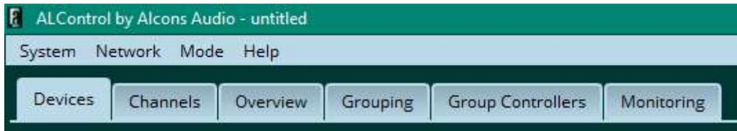
Devices: there are two sections in this Tab: In the *left* section, the discovered (when network on-line) Sentinel devices can be selected into the project; This can be done both with network in on-line or off-line mode. The type of Sentinel can be selected (S3 or S10), as well as output mode configuration (drop-down menu):
